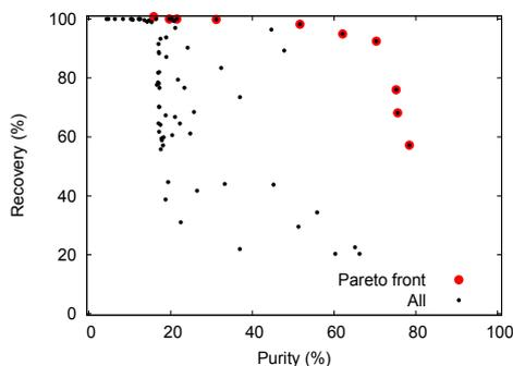
Figure 4. Trade-off of purity and recovery. Here the surrogate-based optimisation required 15 evaluations of the high-fidelity model (above the 64 initial design points)
