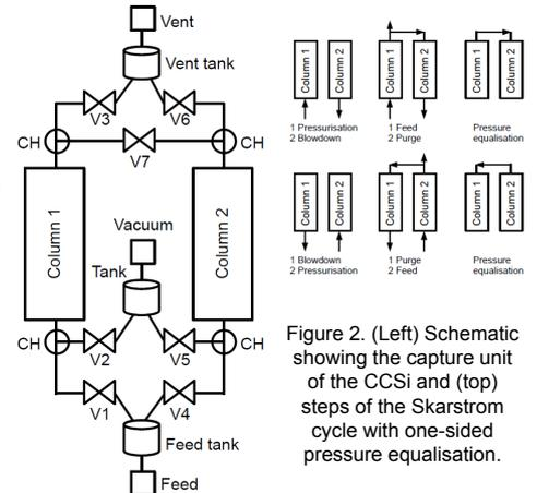
Figure 2. (Left) Schematic showing the capture unit of the CCSi and (top) steps of the Skarstrom cycle with one-sided pressure equalisation.
