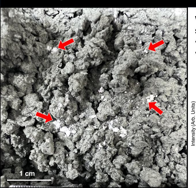
White efflorescence's observed on the surface during initial drying
