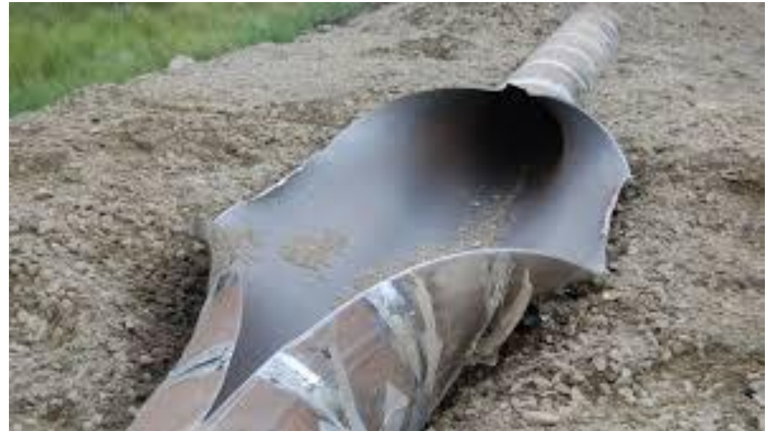
Image from “SINTEF coupled FE-CFD model for fracture-propagation control in CO 2 pipelines”
